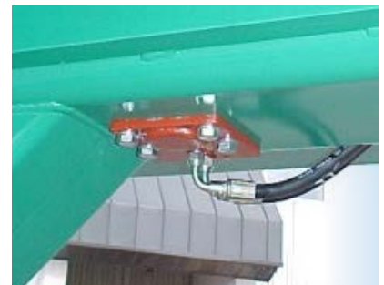
Hydraulic cylinders in the bending deck secure the mat firmly against the mandrel for each bend. The cylinders are accessible for repair or replacement. The photo shows the bending deck and mandrel fully engaged.
