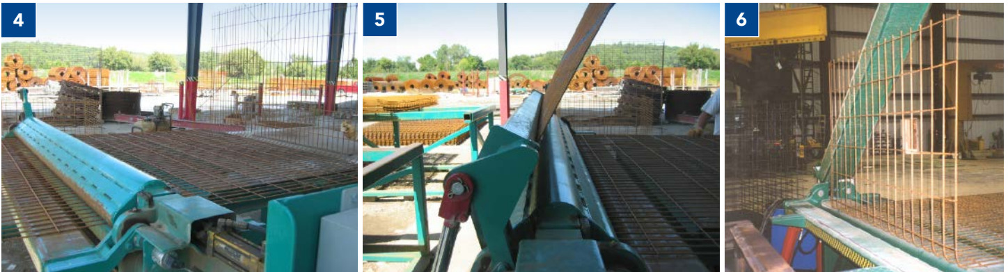
"L" shaped mat is pulled forward and the second bend located.
