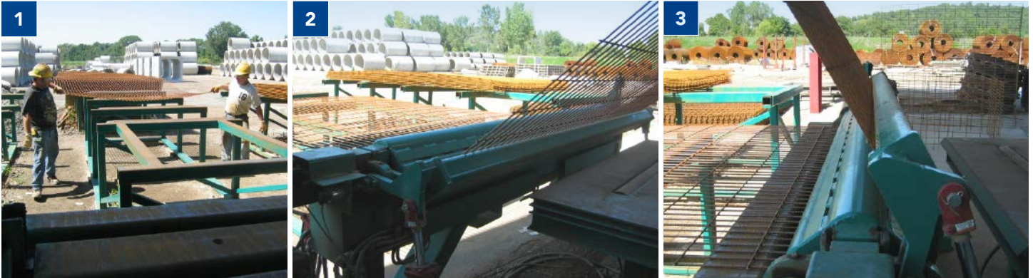
Mat is introduced between the deck and mandrel; and located for the first bend.
