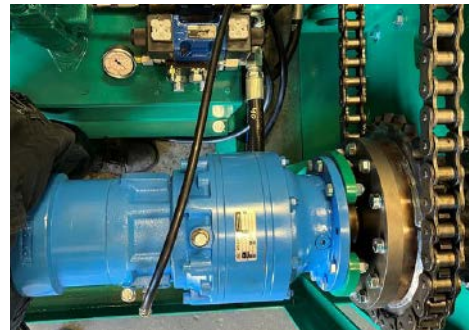
A single drive motor provides all the power required to operate the CMR mesh roller.
