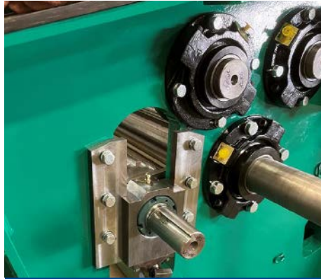
Piloted bearings put the machine rolls in the correct position at assembly. No further adjustment is required.
