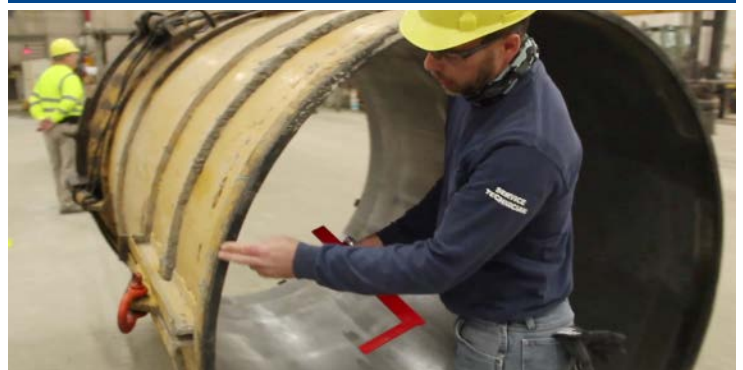
Jacket top inspection
