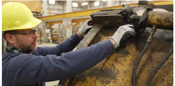
P-Lock assembly inspection
